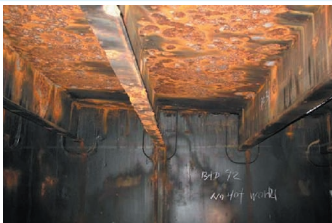
Corrosion in seawater ballast tank
