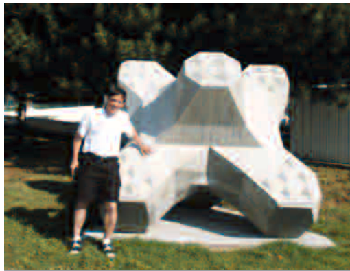
Breakwater construction units (2005)
